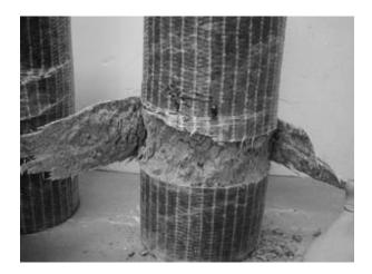
Figure 5. Localized Damage Zone of C1-UC1
