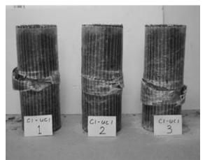
Figure 4. Failure of C1-UC1
