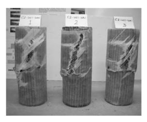
Figure 6. Failure of C2-UC1-WA1
