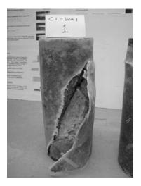
Figure 12. Global Concrete Shear Crack
